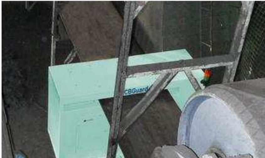
The CBGuard scanner is suited for a belt width of up to 3.2m, a belt thickness of up to 60mm and a velocity of up to 8 m/s
