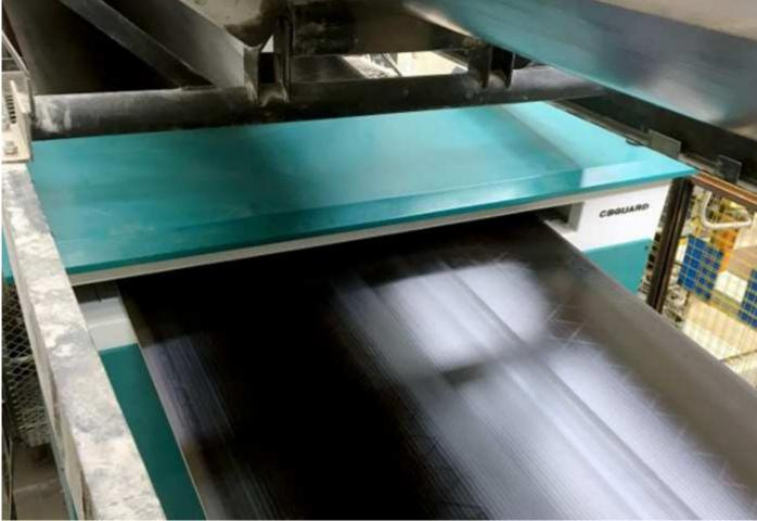
The monitoring technology of the CBGuard system generates a constant video feed of a scan that penetrates the conveyor belt and notifies the operator of problems. Courtesy of Conveyor Belt Gateway
